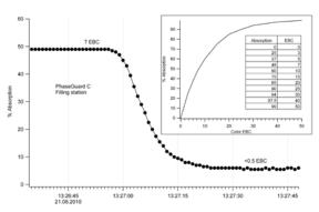
This diagram shows a typical pattern of a phase change from beer to water, which takes place within about 20 seconds. The PhaseGuard C picks up this interface change quickly and with high precision. It allows the user to select the switching point which he believes is the optimum (compromise between beer loss or amount of water in the storage tank).
