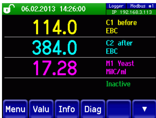
Picture 1: Display of the measurement at the SICON M: „C1 before“ shows the turbidity of the wort before yeast dosage „C2 after“ shows the turbidity of the wort with the yeast added „M1 Yeast“ shows the yeast concentration in Mil. Cells/ml
