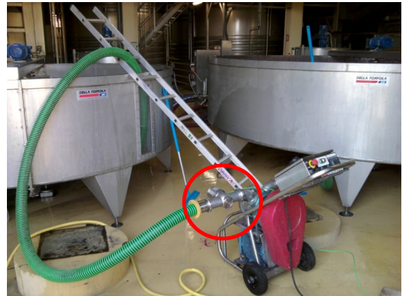
Picture 1: Mounting of TurbiGuard (circle) on a pump trolley
