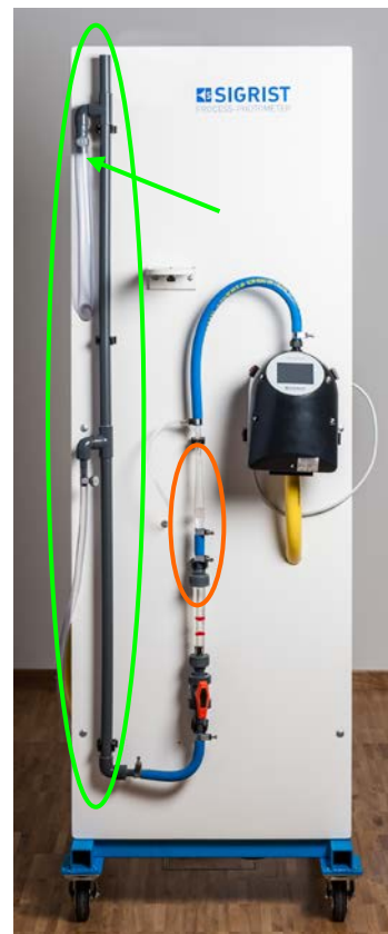
Picture 3: AquaScat with level control and vent pipe
