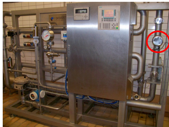
Pict. 2: Example of a blending plant with integrated ColorPlus (circle)
